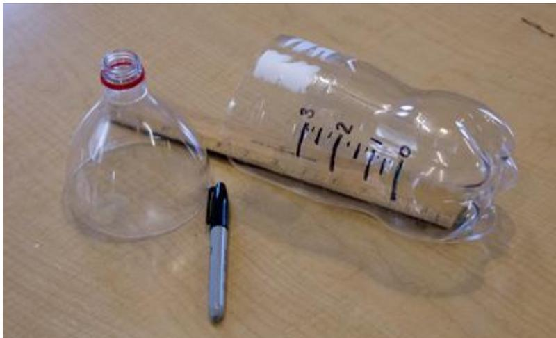
1. Cut the upper part from the transparent bottle as shown. Be sure to ask an adult to help you cut the bottle. Using a ruler, mark the measurement increases starting from about 2" from the bottom. Use millimetres as a source of measurement.
