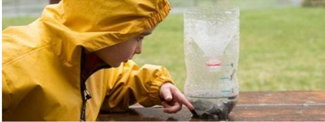
There is no better way to learn about time than to observe it and experience it firsthand. Monitor local precipitation with a simple rain gauge made from a transparent plastic bottle. If you carefully calibrate it, you can take fairly accurate readings.
