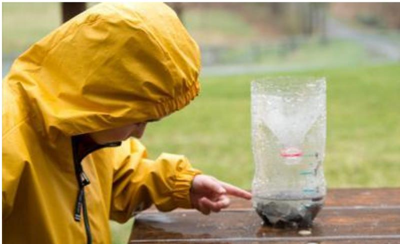
4. Wait for the next rain and observe and record the rainfall. You should leave the rain gauge for either a few days or a whole week and record the amount of total rain collected and how the rain measured the first day and as it added in the second day and so on.
