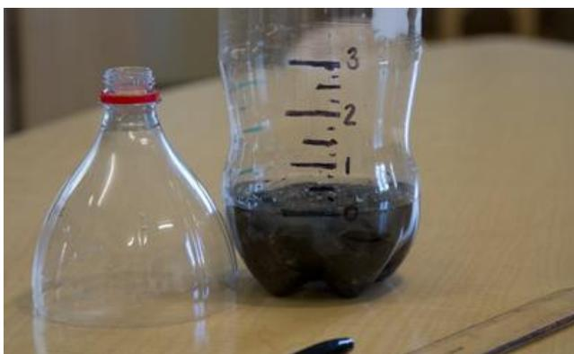
2. Put a few small rocks on the bottom (for weight), then fill the bottle with water up to 0 mark. This will calibrate your gauge.
