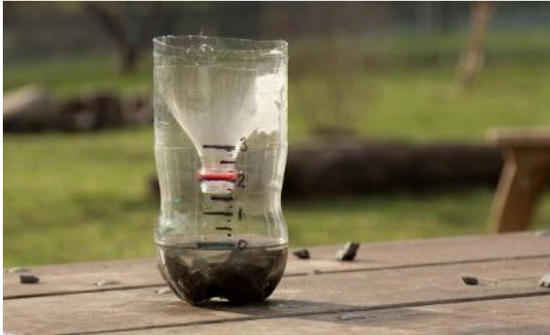
3. Turn the top of the bottle into a rain gauge to act as a funnel. If you need to make sure that the upper sticks are held, use a tape to fasten the funnel of part of the rain gauge. Place the meter on a flat surface from the outside.
